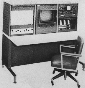
CRT computer-controlled display terminal facilitates man-machine interplay on complex problems requiring human creativity.
